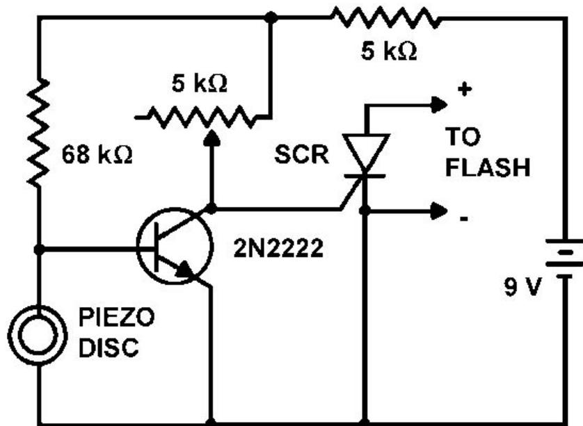
for less than \$10. It consists of a piezoelectric microphone,<sup>2</sup> a general-purpose transistor, a 5-kΩ variable resistor for sensitivity control, a 400-V SCR,<sup>3</sup> and a 9-V source. The SCR must be sensitive to 0.2 ma of gate current or less.
