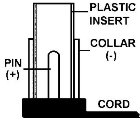
2) Clip the earphone off the earphone cable of the tape recorder. The leads that come from the recorder are the ones that will be used. They should be several feet long to allow the recorder to be positioned far from the flash. If they're too short, splice extra wire onto them. Strip a quarter of an inch of insulation from the ends of the leads. Then wrap one lead (either one) around the gate of the SCR and the other around the cathode. Solder or tape them in place.
