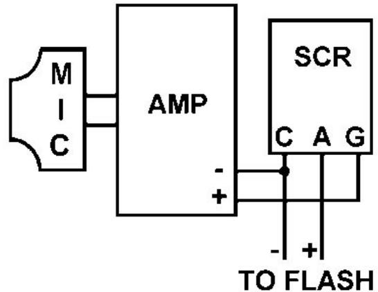
The SCR has a second function. It serves to isolate the amplifier from the voltage across the terminals of the flash unit. This can be as high as 330 V for older flash units. Newer units, however, may have low-voltage trigger circuits. In any case, an SCR rated for 400 V is sufficient.
